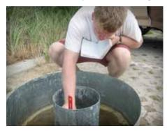
Students can use an infiltrometer (shown at left) to measure surface infiltration as class work.
