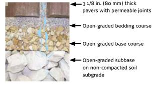
Permeable interlocking concrete pavement (PICP) with open-graded base and subbase for infiltration and storage.
