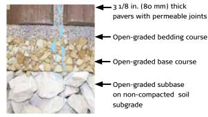
Permeable interlocking concrete pavement (PICP) with open-graded base and subbase for storage and infiltration.
