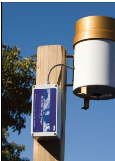
Figure 4-6: Tipping Bucket Rain Gauge with Continuous Wireless Transmission of Data
