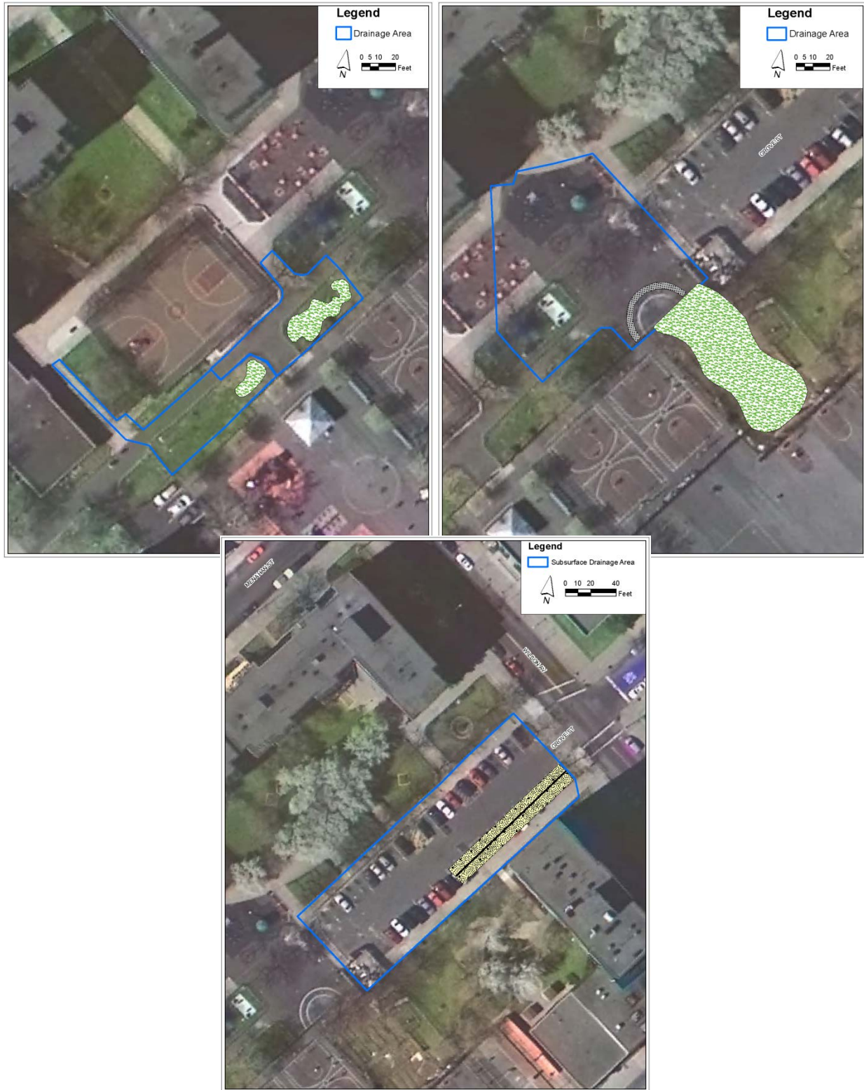
Figure 6: Hope Gardens Drainage Areas and Facility Layout (Hatched Areas) (Clockwise from top left to bottom, the photos show Bioretention 1 and 2, Bioretention 3, and the Subsurface Facility.)
