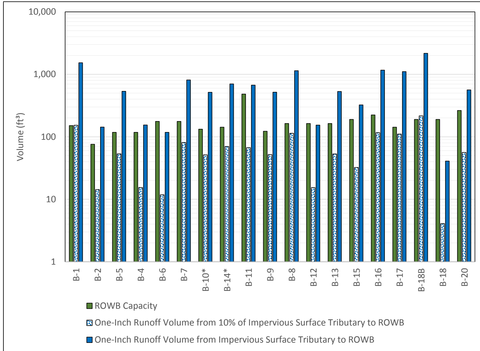
Figure 3-19: Calculated ROWB Managed Volume Capacity and ROWB Sub-Tributary Drainage Area Runoff Volume for 1-Inch Rainfall within Demo Area 3
