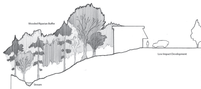
Figure 6-1. Section showing wooded riparian buffer along the downslope side of the LID project
