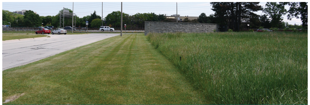
Figure 7.1.3: Some LID retrofit options, like no mow zones will actually reduce your operations and maintenance burden on your property. (Source: CVC)
