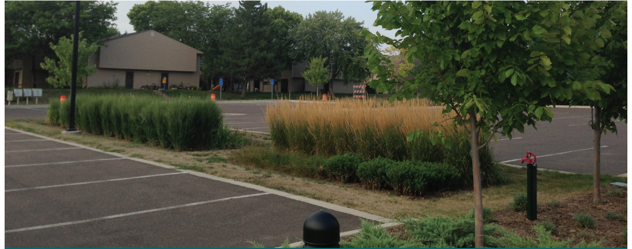
Figure 4.3.1: Green features in your parking lot provide shade and evaporative cooling. This plays a role in reducing air temperatures on your site and making the walk from a car to your municipal facility a better experience during hot summer days. (Source: CVC)
