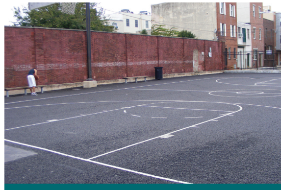
Figure 2.3.2: Porous asphalt can be used in recreational spaces, such as this basketball court. Some applications, like skate parks, are not suited to porous asphalt as the sport requires special pavement to absorb falls and withstand wear and tear. (Source: Aquafor Beech)
