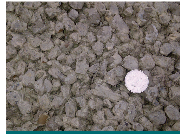
Figure 6.1.2: This photo shows the surface texture of pervious concrete. This surface is slightly rougher than conventional pavement and provides excellent traction. Most pervious concrete products are compliant with provincial accessibility standards. (Source: Aquafor Beech)
