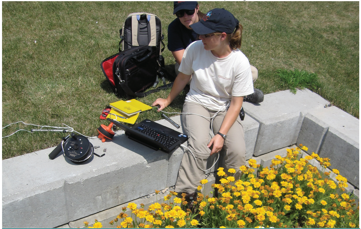
Figure 7.5.2: The water level logger has been pulled out of the bioretention cell observation well. The water level data from the logger is being downloaded directly to a laptop before being put back in the well. (source: CVC)
