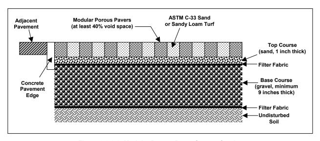
Figure 3.3.8-2 Modular Porous Paver System Section
