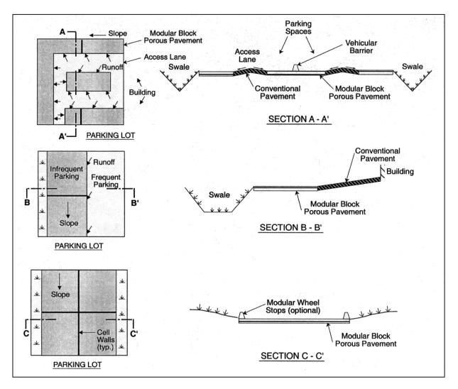
Figure 3.3.8-3 Typical Modular Porous Paver System Applications (Source: UDFCD, 1999)
