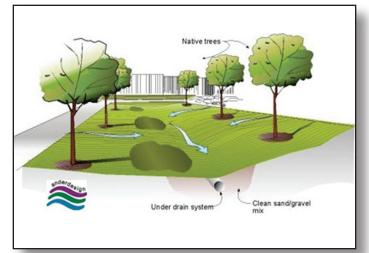
Figure 2.5b Bio-swale Schematic Image Courtesy of: Pierce County WA and AHBL, Inc.
