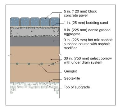
gram). The asphalt subbase included drain holes to allow movement of water through the aggregate base, asphalt, select soil subgrade, and into a drain system routed to the storm water drain pipes.
